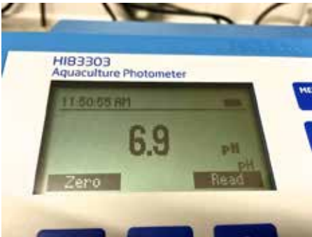
Top: Hanna Instruments bench Aquaculture Photometer showing KH reading. Bottom: pH reading.
