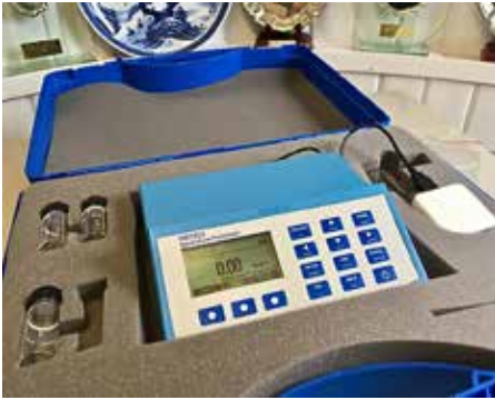
HI-83203 Aquaculture Bench Photometer used as a double check to the in-line system.
