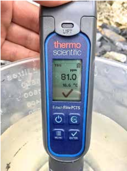
Thermo Scientific Meter used to measure Total Dissolved Solids (TDS).
